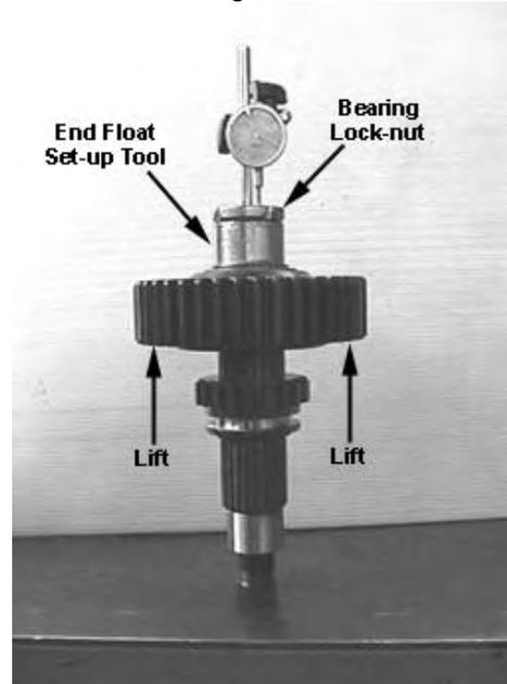
6. Gear end-float should be .000 to .002 inches **loose** (see page 8). If the end-float is not within the specifications the gear and rear bearing will need to be removed and a bearing spacer of a different thickness used.
