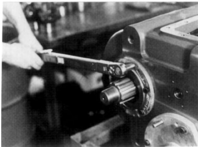
FIG. 6.2-9 Tighten cap screws to specified torque. Adjustment of bearing end float will be discussed in later section.
