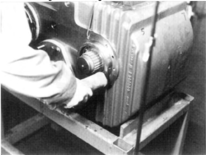
FIG. 6.4-7 Allow bearing to cool and tap bearing cup into housing bore.
