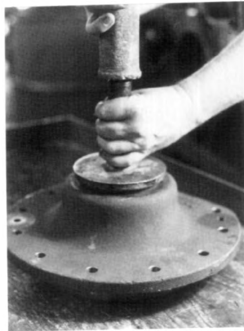
FIG. 6.4-14 Seat oil seal in speed carrier.
